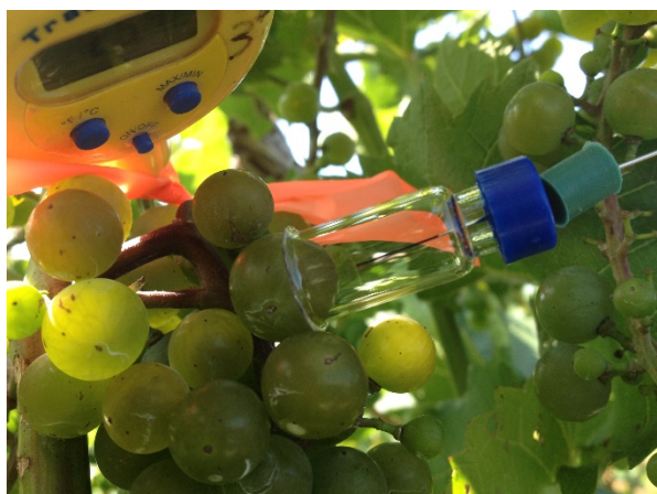
Figure 1. Sampling of volatile emissions from La Crescent grapes. A 2 mL glass vial with modified open and flared bottom was fitted with Teflon septa and screw cap (blue) was placed on a maturing grape. A slight vacuum was pulled using a 10 mL syringe and needle. A SPME fiber was inserted, and exposed for 30 minutes to collect volatiles in-situ (seen inside the vial as a black 10 mm long and ~0.3 mm diameter fiber). SPME fibers with collected volatiles were stored in cooler, transported to laboratory, and analyzed at Iowa State University using multidimensional gas-chromatography-mass spectrometry-olfactometry.
